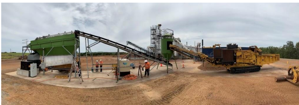
Woodchipper (right) feeds the screener (left) which ensures woodchip sizing is optimal for the plant
