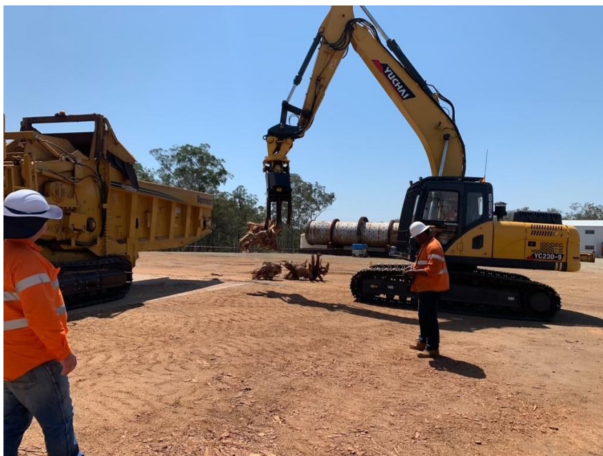
Wood handling excavator feeds stumps into the chipper
